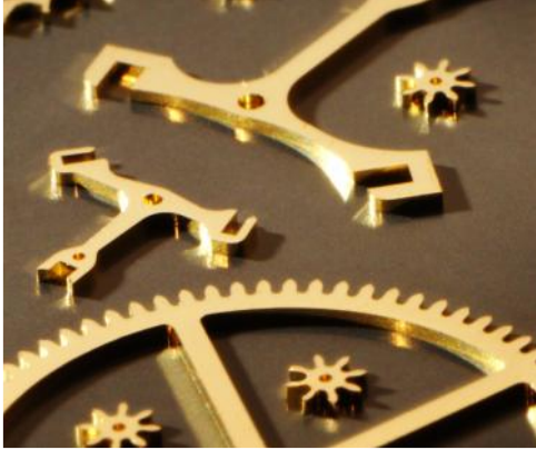
LIGA parts made of gold; the diameter of the smallest parts is near 1mm
